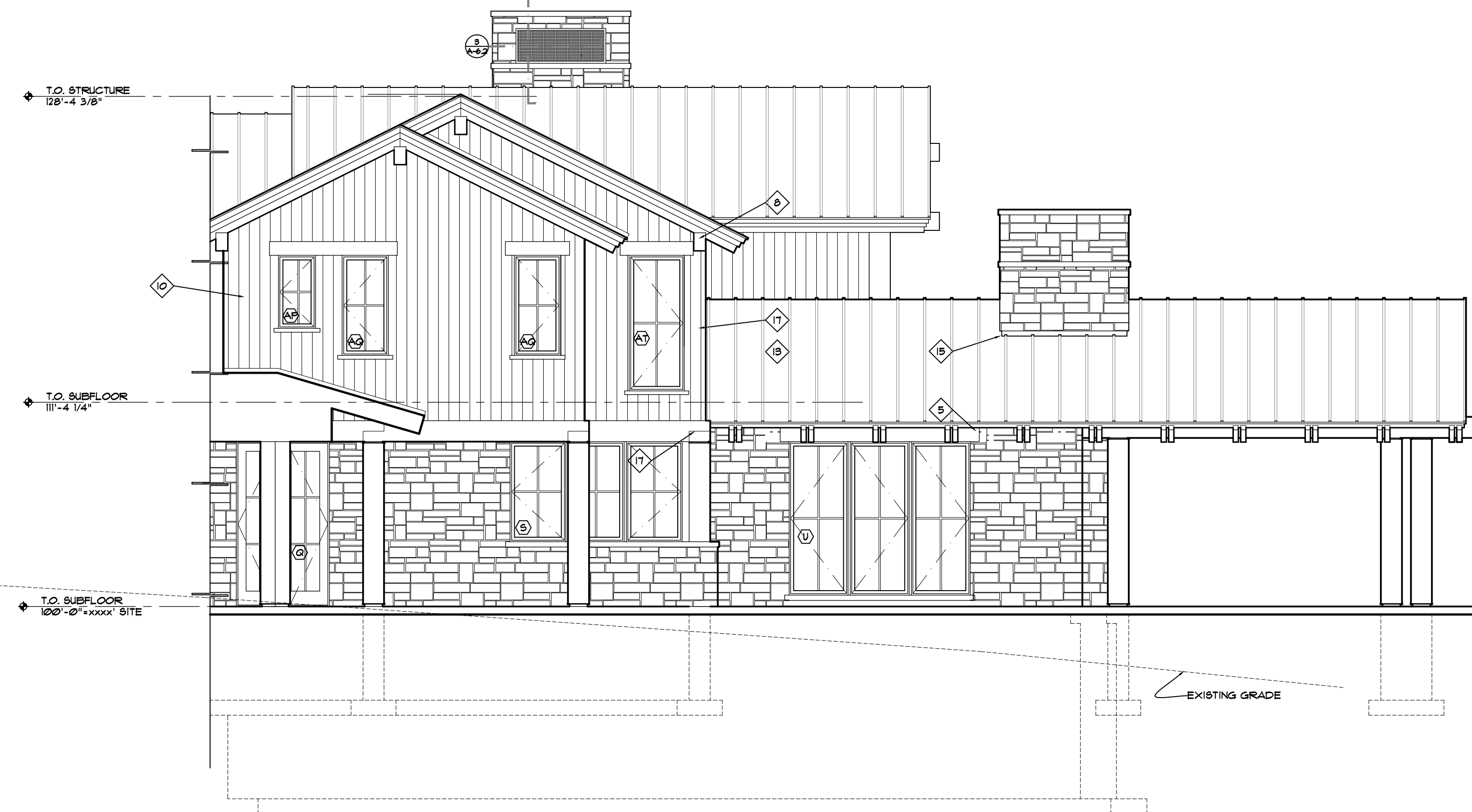
G PARTIAL EAST ELEVATION @ TERRACE / FAMILY ROOM 3/16" = 1'-0"
